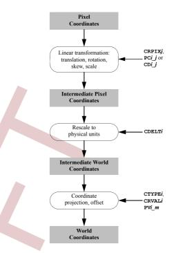
Fig. 2: A schematic view of converting pixel coordinates to world coordinates.
